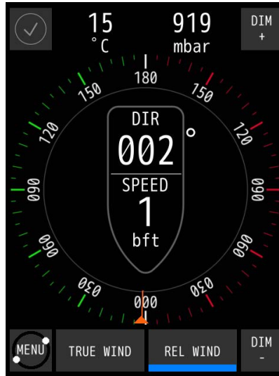
Figure 18: Main Screen AlphaMeteo Aft
