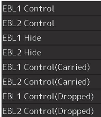
**2 By turning the dial, select either [EBL1 Control (Carried)] and [EBL1 Control (Dropped)] or [EBL2 Control (Carried)] and [EBL2 Control (Dropped)].**
