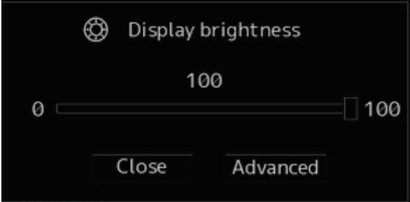
It is possible to adjust the brightness of the display section by rotating the [MULTI] dial.
