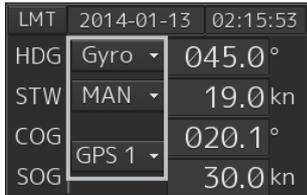
Select the sensor source in the [Source] combo box. The following sensor sources can be selected. When [Menu] is selected, the [Sensor Selection/Status] dialog is displayed.
